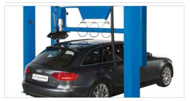
Contour controlled, rotating high-pressure roof beam reaches all places close to the vehicle
