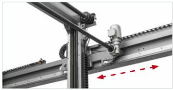
$\, {\color{red} {\bf 7}} \,$  Linear drive and guide on the lifting frame and travelling beam.
