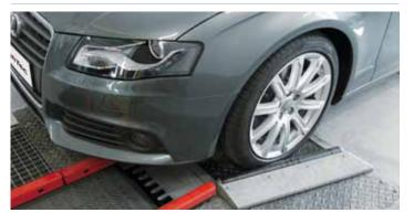
Travelling plate on roller bearings facilitates entry by inexperienced drivers and manoeuvres the vehicle on to the conveyor.
