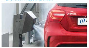
Swivelling point jet nozzles move back and forth over the vehicle for effective precleaning on all vehicle sections.
